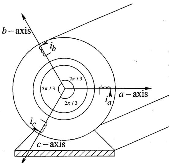
In the airgap, the a-b-c sequence causes the flux-density distribution to rotate counter-clockwise. Therefore, the induced voltage in phase-a peaks first, then  $\omega t (= 120^\circ)$  later in phase-b (which is placed  $120^\circ$  ahead physically, compared to phase-a).
