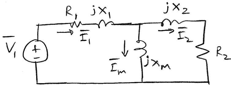
$$\begin{aligned}\bar{V}_1 &= \sqrt{2} \times 120 \angle 0^\circ \\ R_1 &= 0.3 \Omega \\ X_1 &= 0.5 \Omega \\ X_m &= j15 \Omega \\ X_2 &= 0.2 \Omega \\ R_2 &= 7 \Omega\end{aligned}$$
