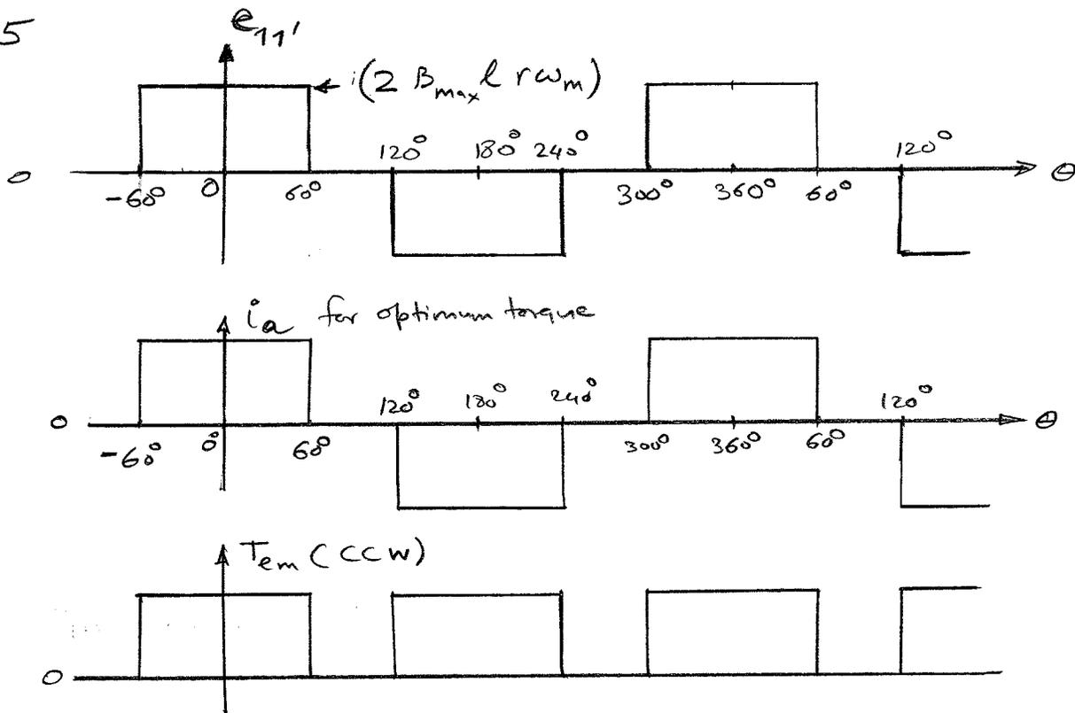
Notice that the torque waveform is pulsating (there is no way to avoid that in this structure); however it is always in the same direction.
