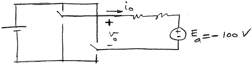
The machine goes into regenerative braking mode while rotating in the reverse direction. Therefore, with the direction for  $i_0$  shown above,
