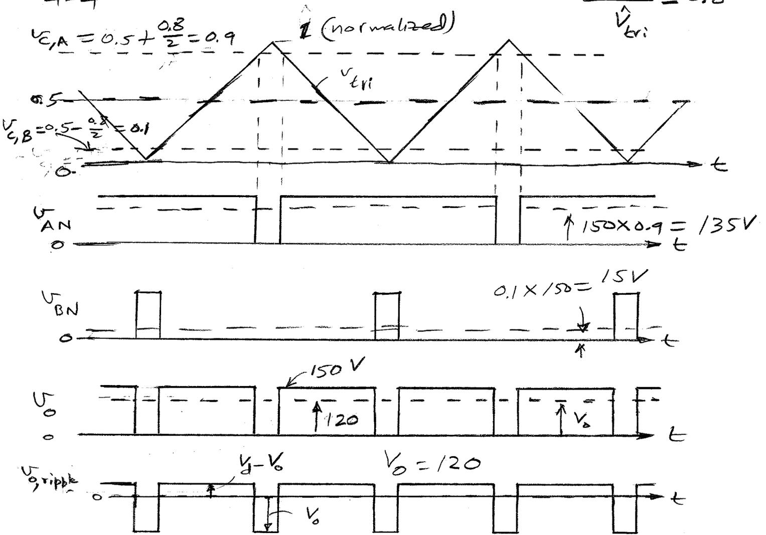
$$V_o = \frac{V_c}{V_{\text{tri}}} V_d = 0.8 \times 150 = 120V$$
