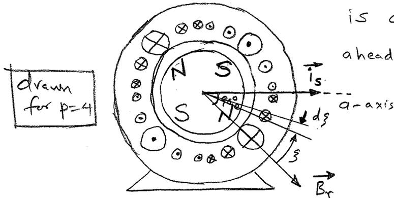
A 4-pole machine is shown below at the instant when  $\vec{I}_s$  vector is along the  $a$ -axis,  $90^\circ$  (electrical) ahead of the  $\vec{B}_r$  space vector in a CCW direction.
